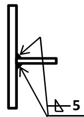
$$\text{Napon u varu } n = Z/A_w \quad n = 150/2 \cdot 0,5 \cdot 23 = 6,52 \text{ kN/cm}^2 \quad \text{M} \dagger_{w,dop} = 12,0 \text{ kN/cm}^2$$
