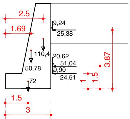
$$\Sigma E_{AV} = 9,24 + 20,62 + 9,90 = 39,76 \text{ kN/m}$$
