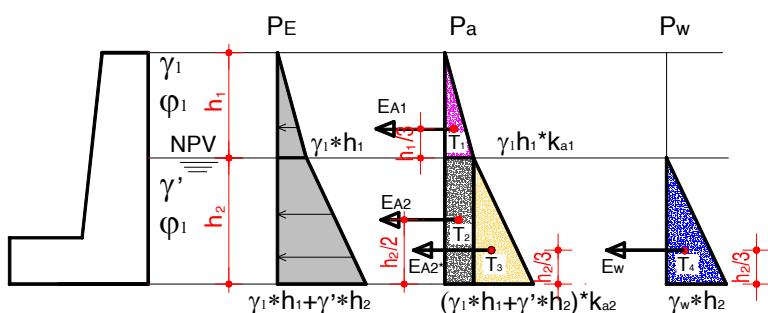
$$E_{a1} = \gamma_1 \cdot h_1 \cdot k_{a1} \cdot \frac{h_1}{2} = \gamma_1 \cdot k_{a1} \cdot \frac{h_1^2}{2} \quad E_{a2} = \gamma_1 \cdot h_1 \cdot k_{a2} \cdot h_2$$
