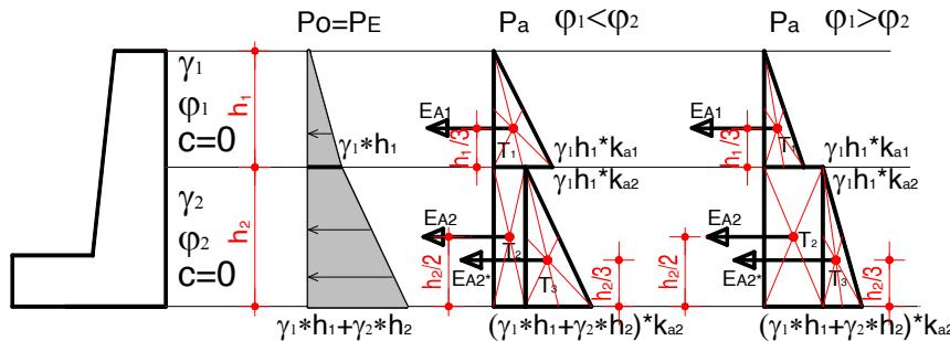
$$E_{a1} = \gamma_1 \cdot h_1 \cdot k_{a1} \cdot \frac{h_1}{2} = \gamma_1 \cdot k_{a1} \cdot \frac{h_1^2}{2} \quad E_{a2} = \gamma_1 \cdot h_1 \cdot k_{a2} \cdot h_2$$
