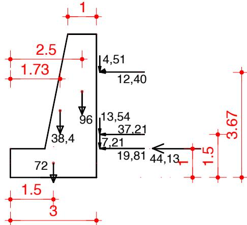
$$\Sigma E_{AV} = 4,51 + 13,54 + 7,21 = 25,26 \text{ kN/m}$$
