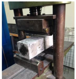
Figure 5: Testing of the flexural strength
